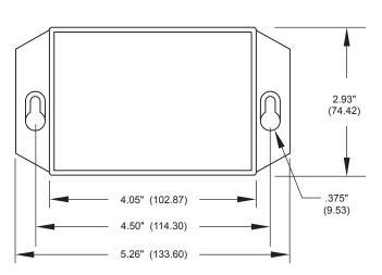
The Model 235P PumpSaver®Plus is designed to protect single-phase pumps from dry-well, dead-head, jammed impeller and overvoltage and undervoltage conditions. The PumpSaver®Plus Model 235P protects 5-15 hp, 230V pumps.
