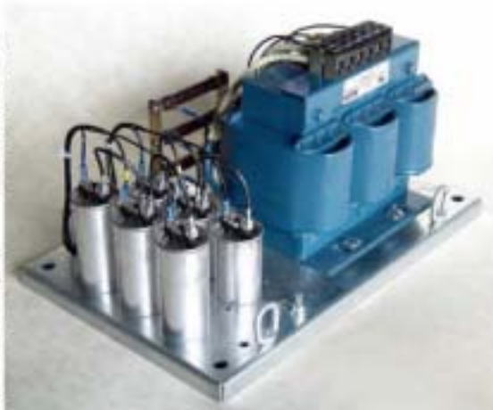
Sine Wave Filters help eliminate the high dV/dt associated with inverter output waveforms in applications where the distance between the motor and the inverter is up to 15,000 feet.
