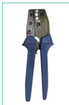
Multiple Crimp Cavities Cat. No: 3057.0 AWG Wire Size: 8,6,4 mm 2 Ferrule Size: 10, 16, 25
