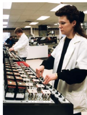
Multiple position testers are used to check the time delay of each timer and timing module. Shown is a pre-encapsulation test.
