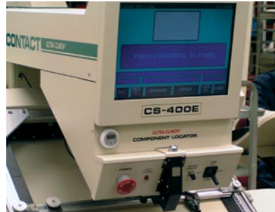
The CS400 line shows the operator where to insert a through-hole component; then clinches the component into position, ready to be soldered.
