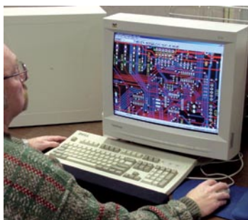
A drafting engineer uses CAD software to design a printed circuit board layout.
