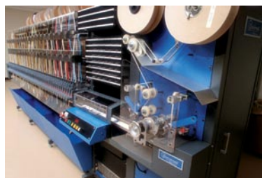
An Axial Sequencer places components in the correct order on a multiple component reel by selecting parts from numerous single part reels.
