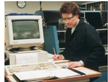
Computers control the operation of the automatic insertion machines. The operator loads a new program as each new job is started.
