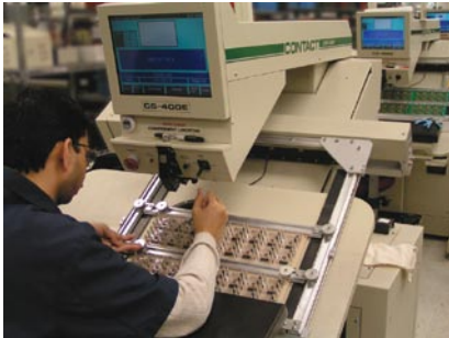
An operator adds components that cannot be automatically inserted.
