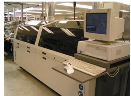
A computer controlled line provides consistent quality soldering of single and double sided PC boards.
