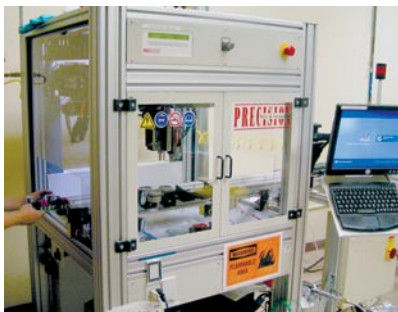
Sensitive electronics must be protected from harsh industrial environments. An automated spraying line ensures uniform coverage of electronic components with clear conformal coating.
