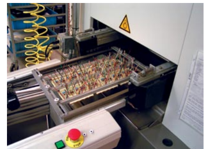
Panels enter the wave soldering line.
